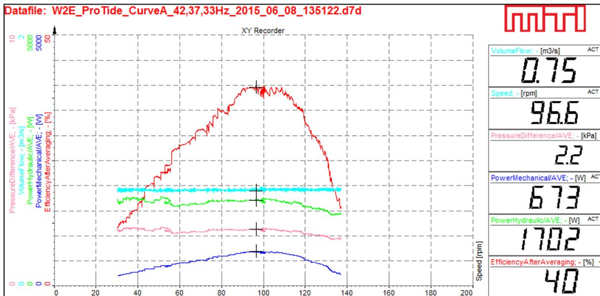
Figure 3.2 Measurement data and relevant calculated parameters of test condition II (0,75 m<sup>3</sup>/s)
