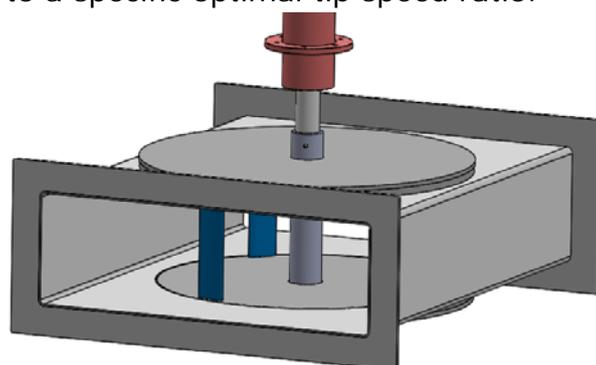
Figure 2.3 W2E's vertical axis turbine, with in blue the runner blades. Not visible is the blade pitch control mechanism.
