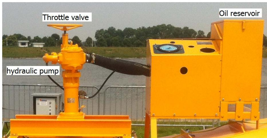
Figure 2.7 Hydraulic braking system
