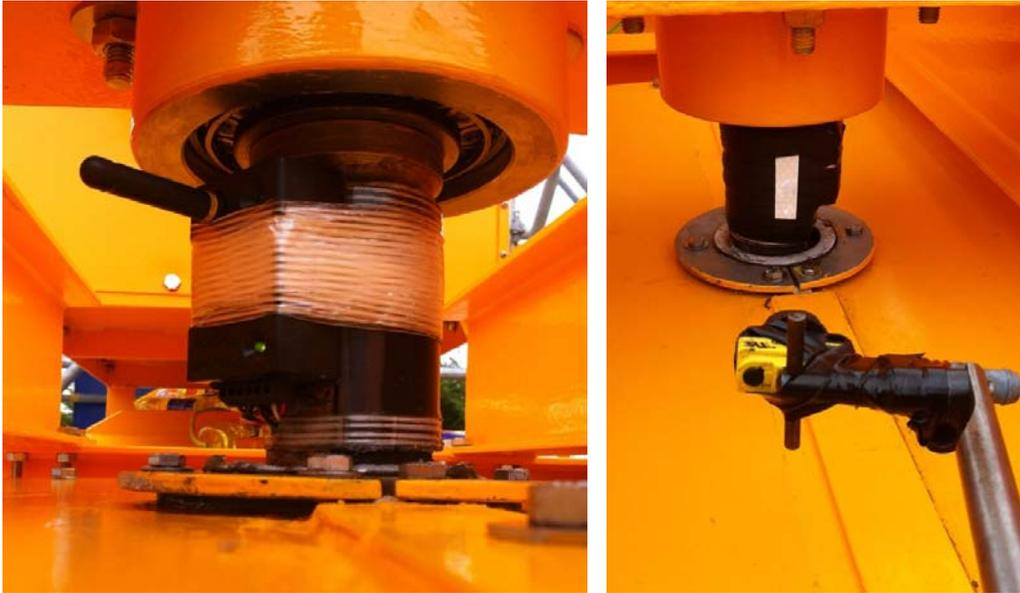
Figure 2.4 W2E's vertical axis turbine shaft measurements: Left Torque sensor with strain gauges and wire-less transmitter and right: optical shaft speed meter.
