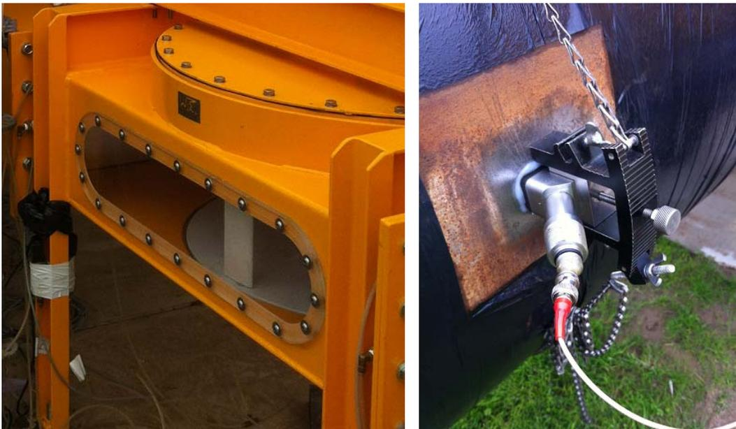
Figure 2.5 Hydraulic measurement equipment: Left: pressure transducers for static pressure across the turbine and right: one of the Ultrasonic flow transmitters/receivers attached to the DN1000 supply tube.
