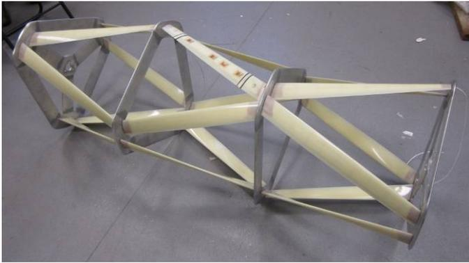
Fig. 1 The 3-bay truss THAWT turbine.
